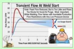
Low pressure devices like the "Gas Guard" tested, eliminate the key feature built into all quality MIG flow control devices since the 1950's, "automatic
