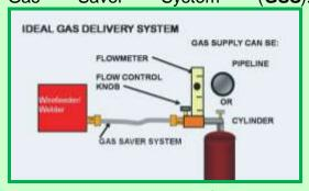
This system will work for any gas supply. The benefits include being able to see the actual gas flow while the **GSS** eliminates the excess "gas blast" at each weld start and controls the gas surge peak velocity improving start weld quality.
