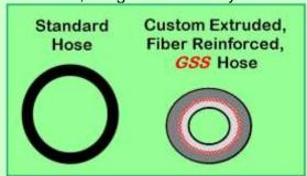
In addition to reduced volume, the **GSS** avoids excess turbulence at the weld start. It accomplishes this by limiting gas surge flow rate using a built-in surge orifice in the feeder/welder hose end fitting. Note: the surge-limiting orifice **does not** limit setting any "reasonable, non-turbulent" steady state flow, with an existing flowmeter, regulator/flowgauge or at the gas source on pipeline gas supply a fixed orifice or flowmeter.
