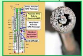
bent, looped and as spatter builds in the nozzle and partially clogs some of the gas diffuser holes. In addition, the gun cable gas passages often doubles as the passage holding the spring wire liner in most MIG gun designs. It may partially clog with wire debris, like copper flakes and lubricant.
