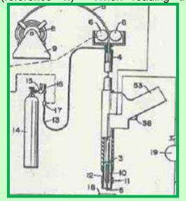
patent teaching it's obvious, some elements required to produce quality welds were missing. One of these missing elements was proper quality gas shielding.
