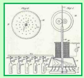
Several sources quote MIG welding as being invented in the 1930's; however, these systems did not work. An example is shown in the figure above from a 1936 General Electric patent (reference 1.) When reading the
