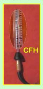
Portable flowmeters operate using basic physics of gas flow. They are accurate and very repeatability. When gas is flowing, a float ball rises in a tapered tube. The gas pressure forces acting on the ball balance gravity as the ball rises. The density of gas must be the into factored the calibration. For welding, measuring the shielding gas exiting a MIG nozzle or TIG cup
