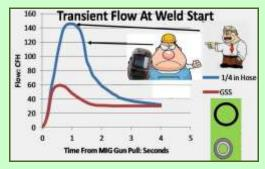
The GSS quickly provides sufficient extra gas to purge the weld start area of moisture laden air at a flow rate that avoids excess turbulence. It quickly reaches the preset, desired gas flow rate. The ¼ inch ID standard hose has peak flows exceeding 150 CFH, which pulls air into the shielding gas stream creating inferior starts and wasting gas.
