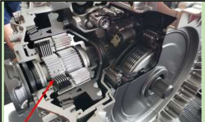
Right eLSD Clutch Pack. Activated with ~3000 psi Using Many Sensors in 0.1 Sec. Locking Both if Commanded.
