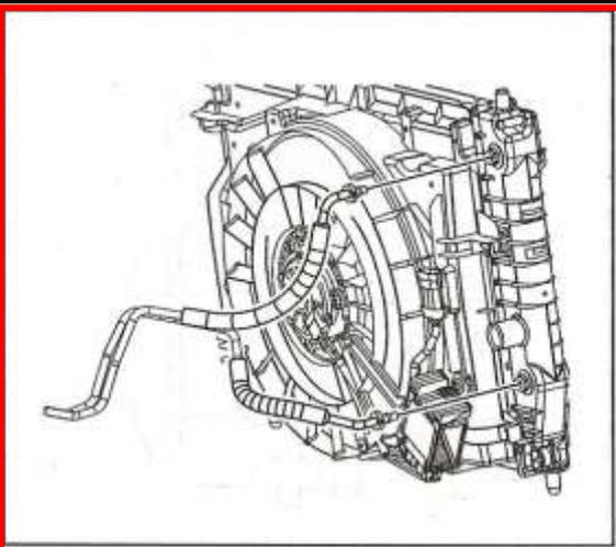
The cooler location for the standard transmission is the same as the automatic but where is the pressure to get the fluid to the cooler? Item 3 in the picture is the pump that is part of the transmission. It turns with the transmission when the car is moving unlike the pump in an automatic that operates when the engine is running.
