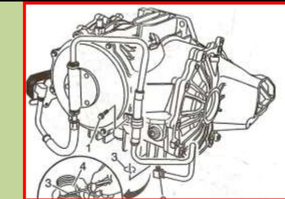
In this view you can see the Differential Cooler detached. It bolts to the left side case cover and the gear oil outlet connects into a “Quick Connect” fitting in the line going back to the differential case. Therefore gear oil comes from the case bottom, is cooled by the transmission oil and returned to the differential.
