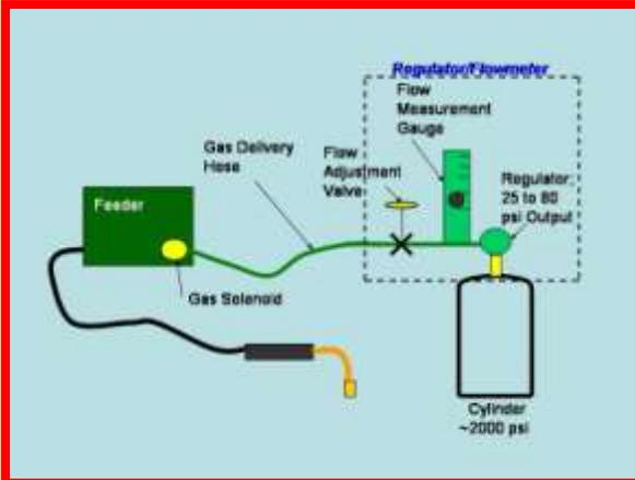
To keep flow at the preset level the gas pressure in the cylinder regulator will be between 25 and 80 psi. Flowgauge regulators (those with a flow calibrated pressure gauge) operate in this pressure range as well.) However to flow shielding gas though the welder and torch typically requires 3 to 5 psi depending on restrictions. Therefore every time
