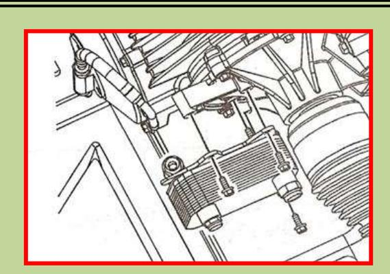
The last of the coolers is one for the power steering fluid. It is a tube and fin unit that sits at the bottom on the radiator and gets cool air from the front of the car.
