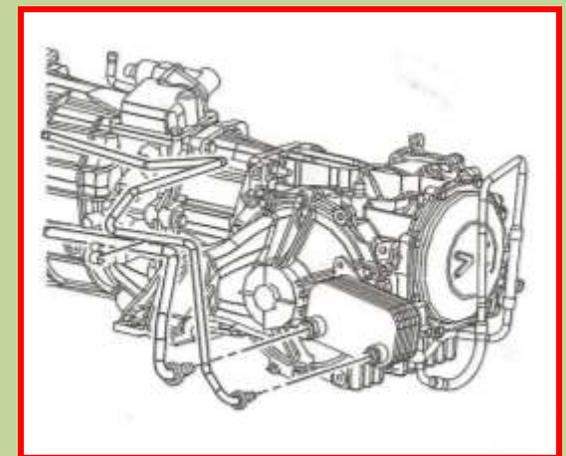
This is a closer view of the Differential Cooler. The return transmission oil line going back to the transmission is shown connected. It basically takes cooled transmission oil (if going through a 200 degree radiator can be called cool) into this liquid/liquid “Cooler” and lowers the differential gear oil temperature if it becomes excessive.
