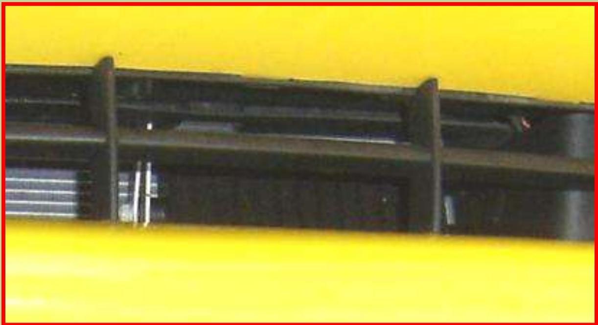
Hard to see this Engine Oil Cooler that is part of the Z51 package? Not surprising it's also hard to find and see most of the extra coolers! The Engine Oil cooler is behind the grill in front of the Air conditioning condenser on the driver side.
