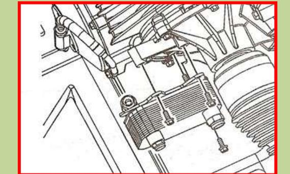
The last of the coolers is one for the power steering fluid. It is a tube and fin unit that sits at the bottom on the radiator and gets cool air from the front of the car.
