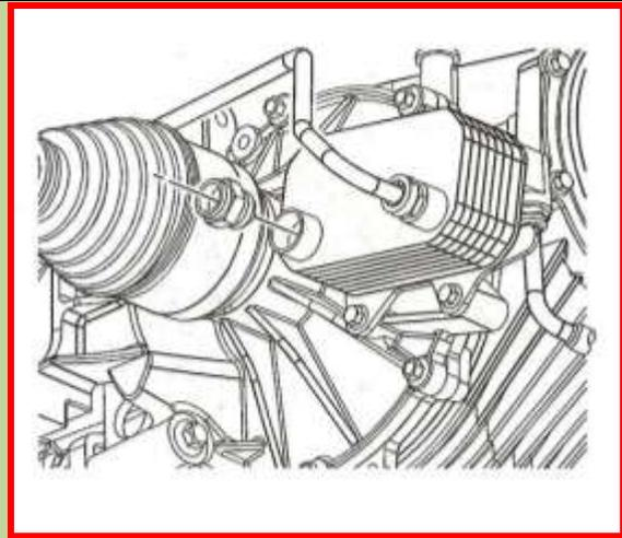
On the Z51 Standard Transmission (and the Z06) the end differential cover includes a gear oil pump. Gear oil is picked up from the bottom of the case (item labeled 2) by the pump and goes into the Cooler. This is done with external lines as shown.
