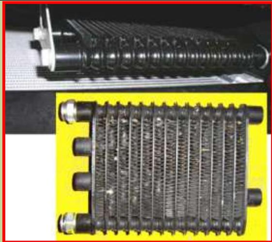
The standard transmission cooler is located the same as the with the automatic, in the passenger side radiator header. Transmission oil enters the top fitting and goes through a cooler surrounded by engine coolant to the bottom fitting where it exits. Where it goes is interesting and we'll discuss with the next cooler.
