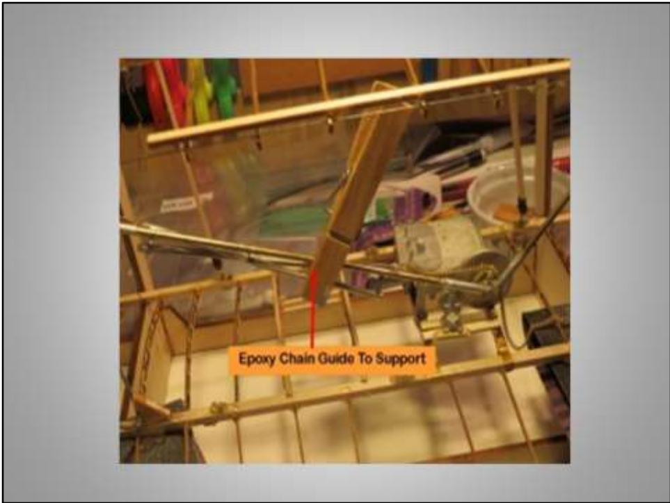
Epoxyed chain guide support to tube.
