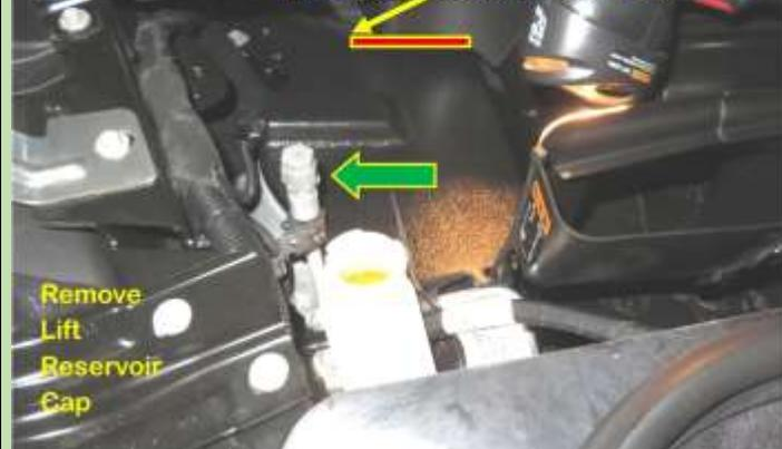
To get the cover past the Lift Fluid Reservoir and some other parts like the "silver pipe" sticking up (Green arrow) you'll have to tilt at an angle. To clear the "silver pipe" I also bent the cover slightly and when past it sprung back. Be sure to remove the red plastic cover over the 3M Tape before you place the cover on.
