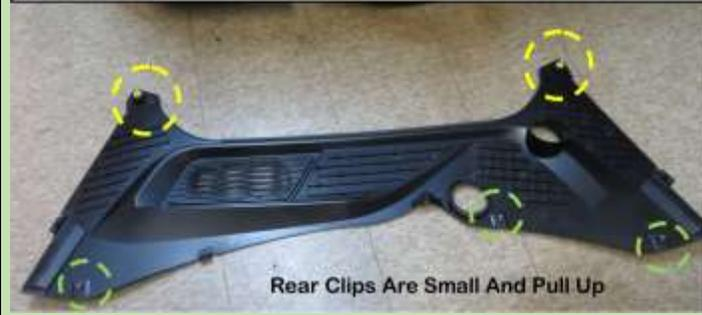
After you remove the two side pieces, the large rear piece is next. First remove the two forward clips made from yellow plastic. The pull straight up. If needed could use a thin trim tool but I found I could get my fingers on the side and pull up. Some have reported breaking these.
