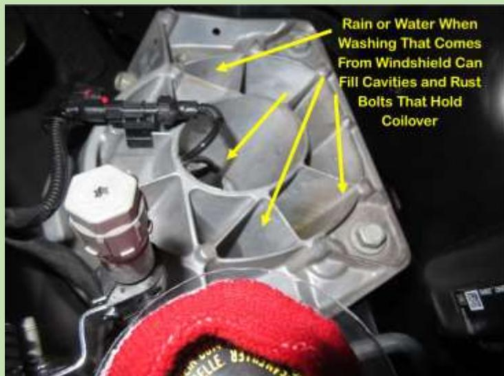
Rain or Water When Washing That Comes From Windshield Can Fill Cavities and Rust Bolts That Hold Coilover
