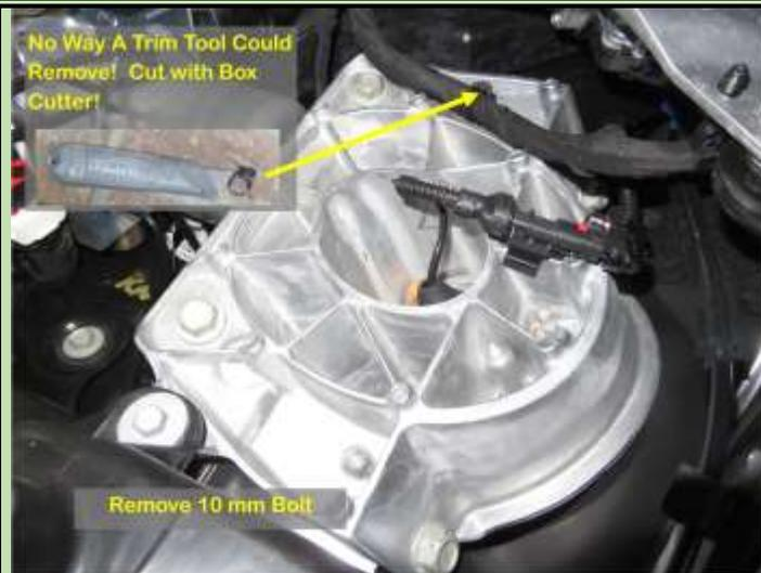
First step on the Driver's Side is to remove the clamp holding a wire bundle. It says use a "forked" Trim Tool. As noted above I have 3 different "forked" ends with different bends. Would not budge! Tried a large screwdriver and it moved a bit, but no way was it coming out!
