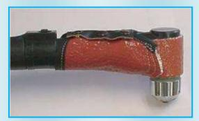
Plasma torches have improved over the years, but it is a simple fact that to build a torch to withstand the occasional heavy gouging abuse would make it heavy and likely not very user friendly. Note the torch on the right with a PLASMIT has seen severe use but is still functional. It would have been destroyed long before if it were not for
