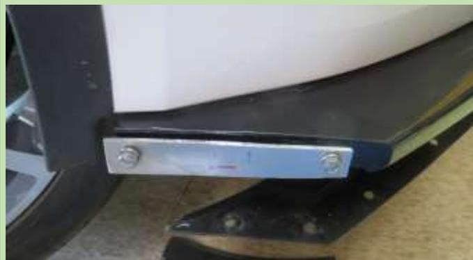
The flat plastic splitter bottom screws were removed to check clearance and since they will be replaced with "Splitter Guards" (more on those at the end!)
