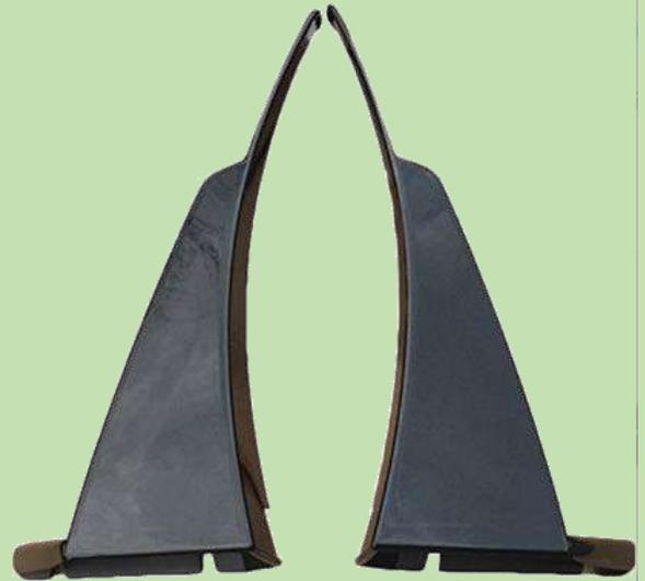
The Stage 2 winglets are held in place with 6 mm visible bolts that are screwed into threads formed in the carbon flash painted, carbon fiber splitter.
