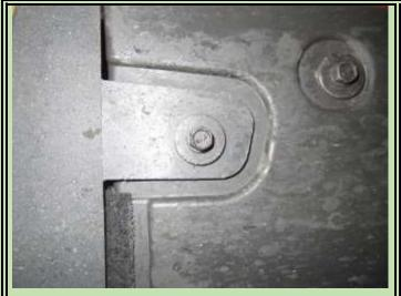
Where the rear splash guard bottom tab inserts into a slot in the body, the front bottom tab does not. It sits in a recess outside the body panel. Not sure why there is a difference, but there is. Both look to function fine.
