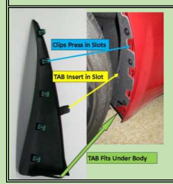
Both front and rear install the same way, this is a picture of the front with an overlay of the splash guard. Not in the instructions, which say align the new clips, you must also put the Tab, yellow arrow, into the slot as you're aligning the clips. Once done simply press the clips into the slots as noted. Does not take much force.
