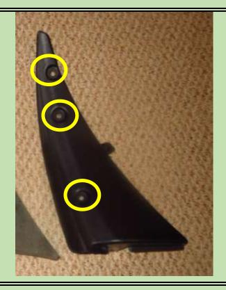
Note the wider, somewhat deeper ASC Frnt Splash Guards do not use the GM clips. You remove tree of the inner fender screws and install the splsh guards using those screws.
