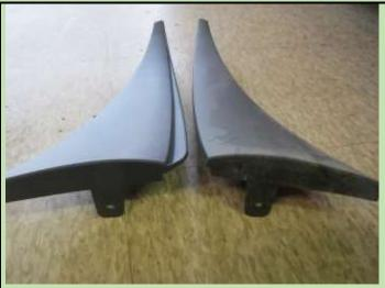
The GM splash guard shape is interesting. The material is very similar to what you'll remove but the extended section is shaped in a clam shell appearance. Not sure why it is contoured that way but although the extension is not as thick as other sections, it looks good. It has a slight raised outer edge for durability.
