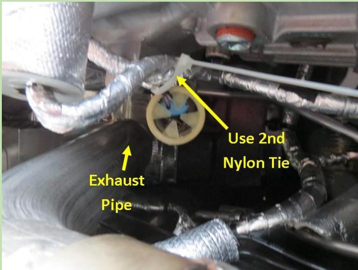
This shows the 2<sup>nd</sup> Nylon tie installed, before trimming the excess tail. Note it pulls the insulated tube covering the Skip Shift Eliminator further way from the exhaust pipe. The bottom of the Skip Shift Eliminator is visible just beyond the plastic tabs at the bottom of the tube.
