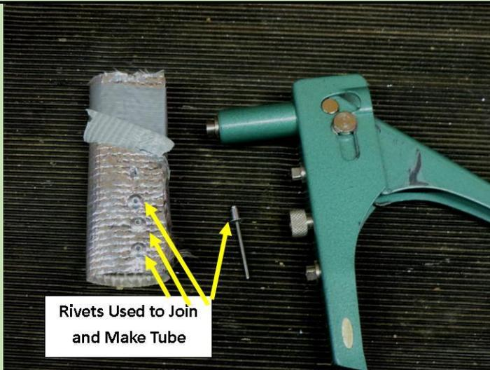
Cut the material and unlike the high temp sealer/glue I used when installing on parts of the street rod (since I did not have any left) decided my seldom used rivet gun would work fine. Used an awl to punch holes into the folded material and the rivet gun make quick work of installing the rivets. Held the shape in place with duct tape that was peeled back as the string of rivets was put in along the seam.
