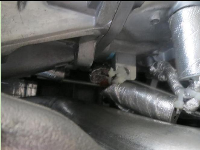
As in the 2104, reach up and unclip the plug from the skip shift solenoid. When removed note the locking tab is on the top. Insert the Skip Shift Eliminator plug in the same direction and it snaps in easily. Note the CAGS Eliminator I purchased came as one part, some are two. The one piece just helps when using nylon wire ties to keep it away from the exhaust.
