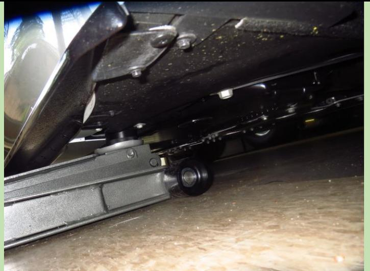
For the C7, the Owner's Manual says to use a jacking pad 2½ inches or smaller. Unlike the 3 inch diameter aluminum jacking pads I used for my C6, there is less room around the "shipping slots" where they fit.
