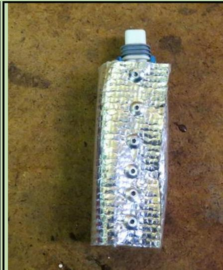
Hard to see the insulated tube over the solenoid connector since it is up rather high on the transmission left side. However the same type of insulation is installed over the temperature sensor that is located near the bottom. The lower one is close to the exhaust pipe and is no doubt why it is used. The wires also have an insulation covering.
