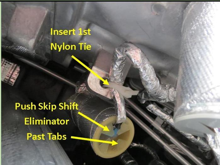
After the connector is installed, be sure to push the Skip Shift Eliminator connector back up into the insulated tube. You'll see there are plastic tabs that hold it in place. Then install a Nylon tie and place it to the side that creates the most space from the exhaust pipe. In this photo you can see on the right, the lower insulated tube that covers the temperature sensor.
