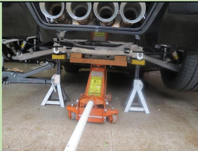
After putting jack pads in the rear shipping slots,, low profile jacks are slipped under and centered under the jack pad. Only needed to raise the car sufficiently to get my large jack under the rea. Note you must have a hard surface. Do not use jacks or jack stands on a soft surface.
