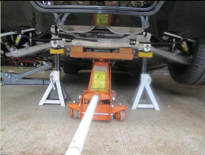
Since I had the left rear wheel removed to install ceramic brake pads, just raised the GS a bit more and put my other large jack with homemade cross brace under the proper spots on the rear cross member. Just follow GM advice about lifting the hollow cast aluminum cross members used on the C7 to reduce the cradle weight 25%.
