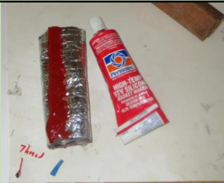
Did not have any of the hi-temp insulation material used for the 2014 C7. Had a less rugged material but when I used the rivets as before they were not holding as well or sealing the seam. However had some Permatex hi-temp RTV that worked well over the rivets,
