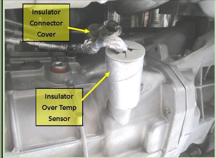
The first step is to cut the existing plastic tie that holds the wires going to both the skip shift solenoid and the temperature sensor. It Chevy apparently asked for a tab to be added to the transmission casting for a plastic tie location. Guess they thought it was essential.
