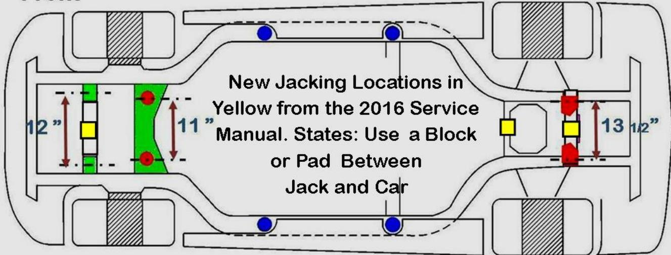
New Jacking Locations in Yellow from the 2016 Service Manual. States: Use a Block or Pad Between Jack and Car
