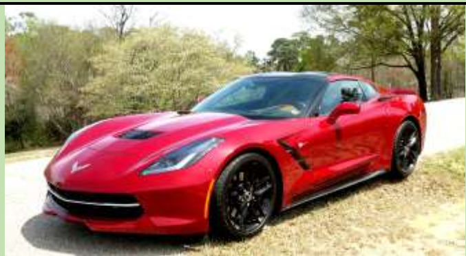
Installed full length side skirts on my 2014 Z51 only using the rivets as recommended
