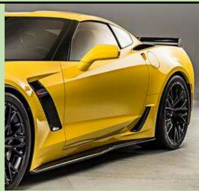
The full-length OEM side skirts on my 2017 Grand Sport were installed with only rivets
