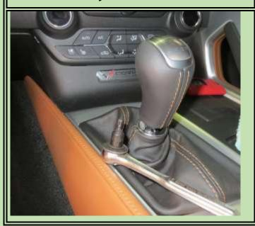
Once the trim ring was pulled down, removing the screw was easier than some instructions suggested. Used a T-25 Torx socket with a ¼ inch drive ratchet wrench. Just placed my right hand on the shifter while turning the wrench with my left. It appeared to have Loctite on the screw but it came turned easily. Some forum comments said to drive the car until the shifter was hot, assume to weaken the Loctite. Thought I might have to heat the screw with a soldering iron tip, but that was not necessary.
