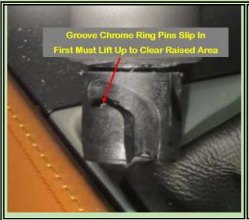
First, with the knob removed you can see the grooves that are on both sides of the OEM shift knob. That is the path two pins attached to the trim ring must follow it have it slide down to reveal the screw holding the knob in place.
