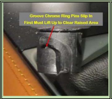
First, with the knob removed you can see the grooves that are on both sides of the OEM shift knob. That is the path two pins attached to the trim ring must follow it have it slide down to reveal the screw holding the knob in place.
