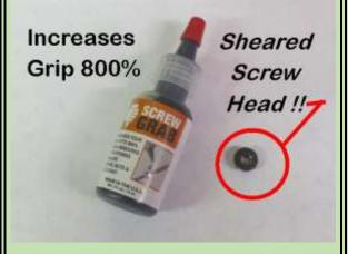
Then placed a drop of this black toothpaste consistence Screw Grip on the Screw-Out!
