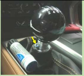
I put blue, medium strength Loctite on the screw that attaches the new knob to the shaft (yellow arrow.)
