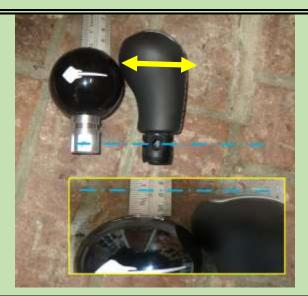
These are the two knobs side by side. Lining up the screw holes and measuring the max height shows about ¾ inches, not a full 1 inch height difference. The OEM knob is 2 inches wide and 2.07 inches front to back.
