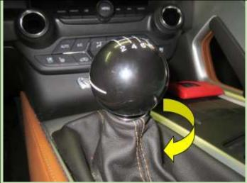
Once the knob is secured, the chrome trim ring is reinstalled. When fully up to the top It required the same arc joint pliers and the friction pad used to remove it, to rotate the ring in the final position. Not the best design especially since it appears it is only made of plastic.
