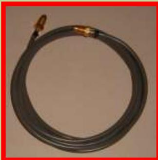
welding stops the pressure in the gas hose raises to the regulator pressure of 25 to 80 psi. That stores up to 7 times the hose volume of gas in the hose. This is similar to your shielding gas cylinder which holds about 150 times the volume of gas as the physical volume of the cylinder due to the high pressure!
