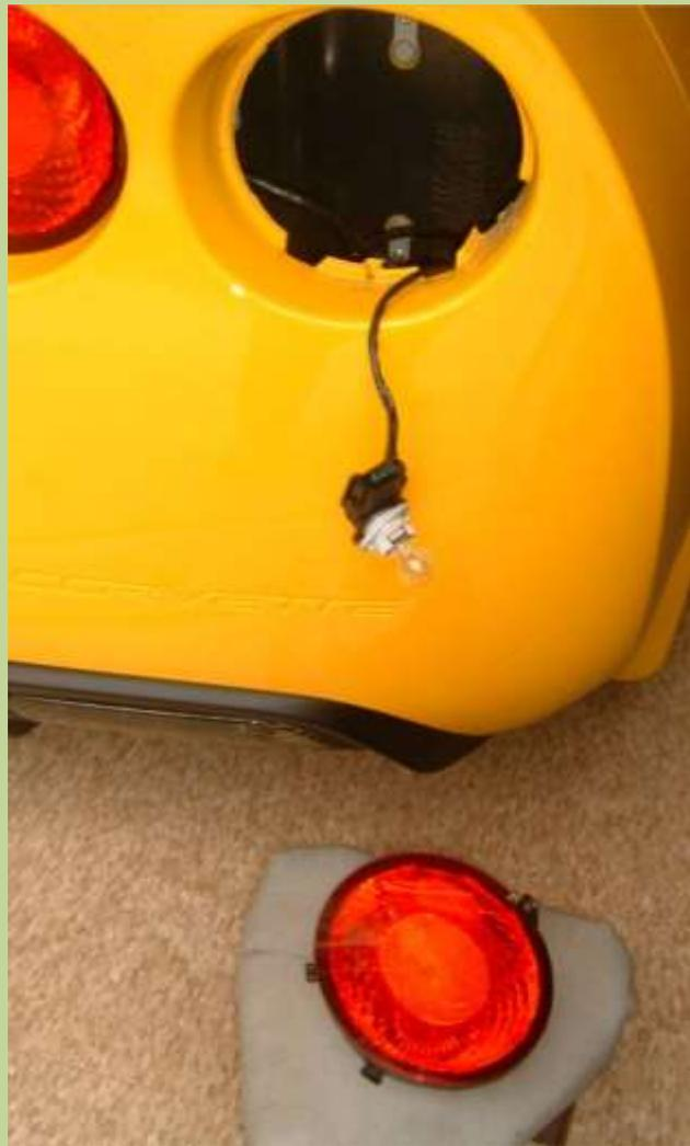
To seal the original socket from water they supply a neat red rubber cover. Simply slip it over the original socket base as they describe and as shown here. It fits over the edge with a modest effort.
