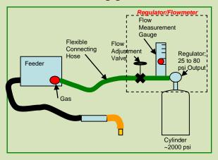
A small restriction orifice or a valve is used to control the gas flow. Typical regulator outlet pressures are from 25 to 80 psi. For CO<sub>2</sub> shielding 80 psi is often used to help prevent ice formation. These higher needed provide pressures to automatic flow compensation for restrictions occurring during use. Anything lower will eliminate this important function (See Reference 3.)
