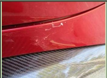
On the first side I moved too far along the side to the front when repositioning myself. This made the angle I was pulling much steeper, perhaps 30 to 45 degrees to the panel. The plastic came off fine but a layer of adhesive stayed on the panel. As I got closer to where I was positioned it returned to an almost perpendicular pull and the adhesive came off with the plastic. Film.
