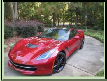
The side skirts installed are made from carbon fiber and sold by LG Motorsports. They are contoured vertically but not horizontally as are the Z06 shirts. They won a SEMA Award when the C7 was introduced. The Z06 has 2 inch wider rear tires so the fenders are wider to accommodate them. For better exit and entry the side skirts are contoured and tuck into the car about where the GM plastic film starts. That is also where your feet plant when exiting.
