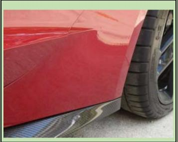
Where I followed the advice of a perpendicular pull 95 to 98% of the adhesive removed with the plastic film. There was little need for a chemical remover. That was the case for most of the second side after I saw what happened in a small area on the first side where I used a much stepper angle!
