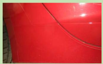
It's difficult to see from pictures how very "noticeable" the plastic "protectors" are that GM installed on the Stingray rocker panels. Especially with time and exposure, the edges become very noticeable as seen to some degree in this picture. Without the addition of side skirts they were needed and protected the panels from small rocks that get thrown from the
