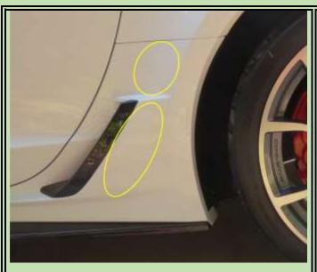
After 18 months no marks on the rocker panels or the lower rear brake ducts that many posts say get marked, perhaps because of the 3/4 standard side skirts.
