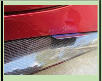
Fortunately, I had only a ~6 inch area along the bottom panel with heavy adhesive remaining. It still took 20 minutes to a half hour to remove all of it! For the remainder of that first side and all of the second side where I only used a 90 degree pull on the film about 10 minutes with the adhesive remover cleaned it all off.
