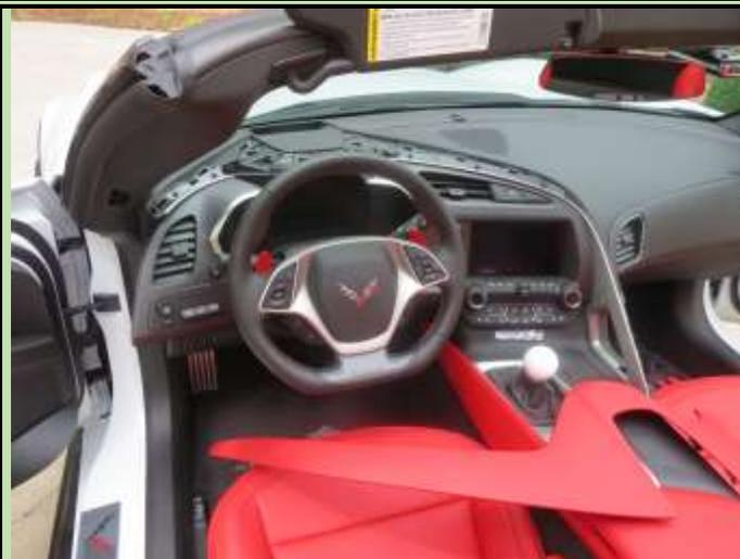
This pic shows the Black upper dash Pad removed and the Red ready to install. Just used the side on my closed fist to tap the clips in place.
