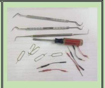
First Step is to pry off the cover behind the mirror. I used a dental pic tool and wedged it in the side of the plastic cover. Have to pull hard but the small clips let go and it comes off.
