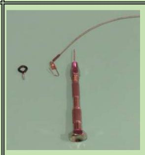
The very thin wire and clasp, from a fishing lure, made a secure safety tether.
