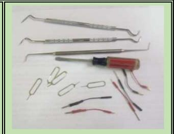
First Step is to pry off the cover behind the mirror. I used a dental pic tool and wedged it in the side of the plastic cover. Have to pull hard but the small clips let go and it comes off.
