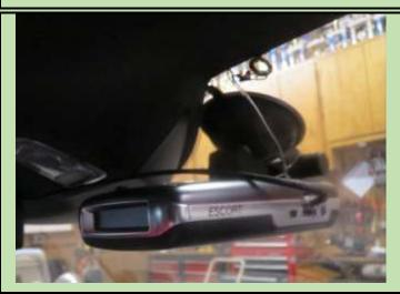
Mounting the detector high on the windshield to the right of the mirror eliminates any obstruction to road vision. The wire routed over the detector and just had enough room.
