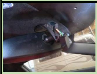
Forum pics were a great help, particularly this one that showed where the Blendmount wires go, in the cable side from the car not that to the mirror. Negative black to Black Blendmount and the Red Blendmount to the purple wire as shown.
