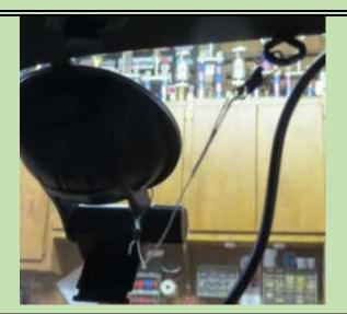
The detector can still be simply slipped off the mount. To remove the mount, you just unclip the fishing leader clamp.
