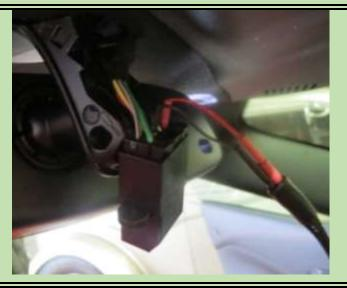
Connected the Blendmount wires into the 15 inch wire then used several wire ties to secure the Blendmount wires to the car harness wires. He pushed the wires up into the area where the car wires go. Thought I would have excess. Did Not. Could have used another 2 inches! As shown in the top pic on this PDF, I used the Escort Passport Mount Sticky Mount.
