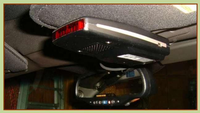
If you want your radar detector out of the way, the best place to install it is with a clip on the passenger visor. The added benefit of that location is you can easily connect to the 12V power available at the mirror. Power is only on when the car is running. (On my '93 Vette spliced into the visor mirror light but this was easier.) If you use the cigarette lighter and a windshield mount the power is always on and if you leave connected for a week a dead battery might greet you!
