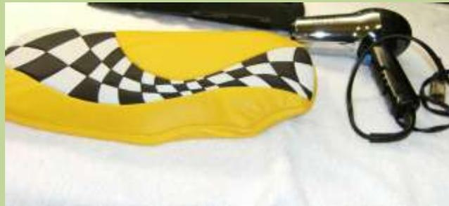
Even if you want to follow their instructions and put the tape in place with the cover off, be sure to fit the cover first and see how much stretching is needed.
