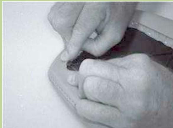
**Pull the material from the center so it stretches over the edge. The stitched edge shows on the outside.**
