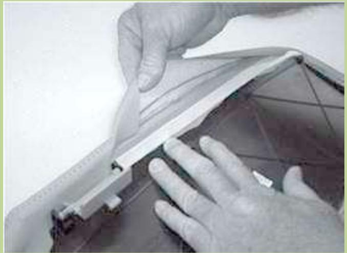
We did put all sections of tape in place leaving the white cover on until we were ready to pull the particular section of cover material an attach it in place. The front corners were the most difficult to stretch to fit so these were pressed on first. Grab the cover as shown and pull it over the corners.
