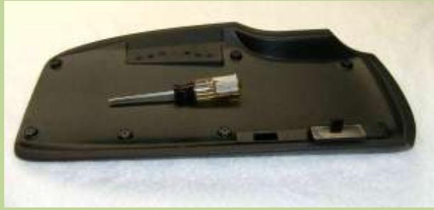
This is a step not covered in the instructions. Place the new cover over the old "BEFORE" you put on the tape. We had to use a hair dryer to stretch it to fit. We worked off the bench and pulled and tugged and the tape would only have gotten in the way. Spent perhaps 15 minutes heating and stretching until the fit was right. Tight but right!
