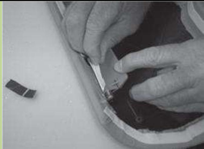
We first attached the cover to the small 1 ½ inch tape under the latch. We pulled hard to get it to go behind the latch. Then we placed the tape under the cover by lifting it up. We found it was easier to apply the tape by cutting rather than bending it at the corners. This also gave us a bit more length of tape- which we needed. Be careful they barley give you enough tape to cover the perimeter!
