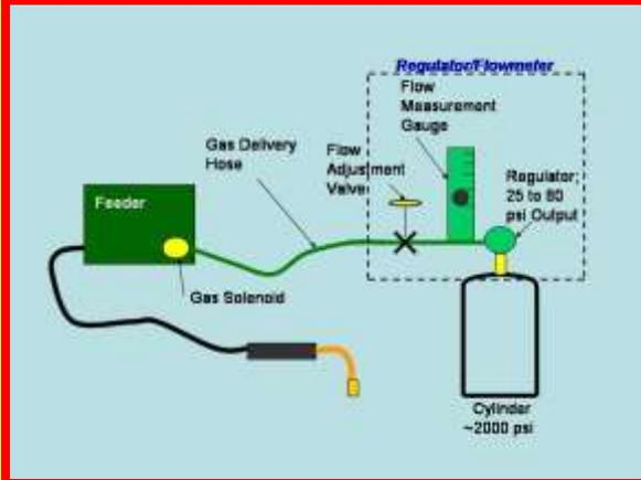
gauge) operate in this pressure range as well.) However to flow shielding gas through the welder and torch typically requires 3 to 5 psi depending on restrictions. Therefore every time welding stops the pressure in the gas hose raises to the regulator pressure of 25 to 80 psi. That stores up to 7 times the hose volume of gas in the hose. This is similar to your shielding gas cylinder which holds about 150 times the volume of gas as the physical volume of the cylinder due to the high pressure!
