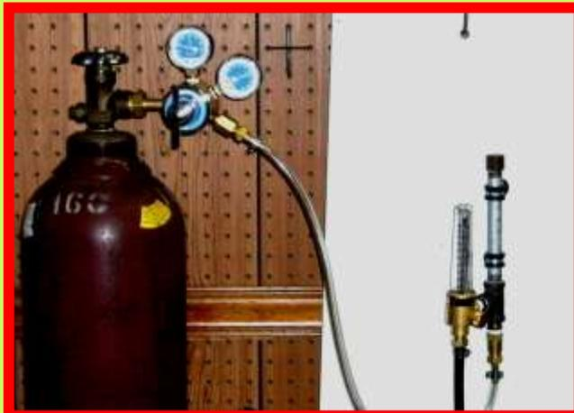
The Victor FM372 flowmeter was mounted on a test pipeline that is supplied from a 75 psi maximum delivery pressure inert gas regulator on an Argon/CO<sub>2</sub> shielding gas cylinder.
