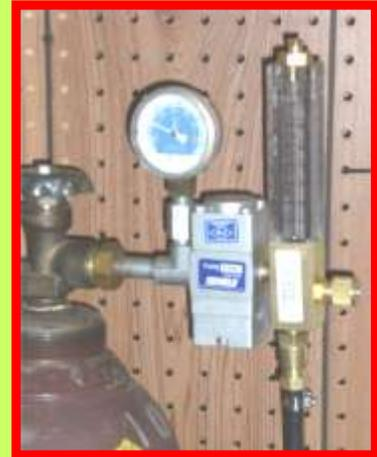
To validate the accuracy of the flow readings of the WAT-PFM, a calibrated regulator/flowmeter was placed on the shielding gas cylinder (picture right.) Flow readings were compared at the end of a hose attached to the flowmeter. Within the precision of our readings, the WAT-PFM read the same flow as the calibrated flowmeter from 20 to 40 CFH.
