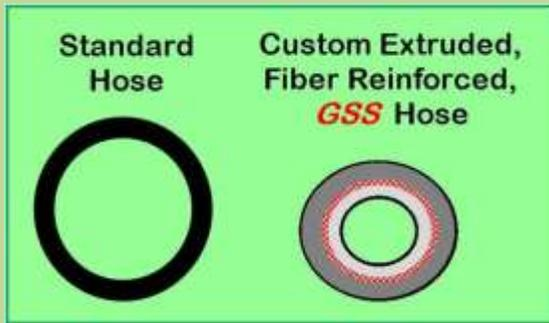
in the **GSS** not only adds to waste reduction, it improves weld starts. The start surge flow restrictor is sized so it *does not* limit normal gas flow settings.
