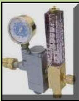
Flowgauge/Regulators (photo left) operate by setting a pressure above a critical orifice. For most MIG shielding gas flow rates the pressure exiting the control orifice when welding stops will range from 40 to 70 psi.
