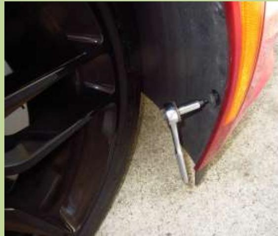
The OEM screw includes a captive washer. The supplied snaps do not. Since the fender liner is only plastic decided to remove the OEM washers and put them on the supplied snap.
