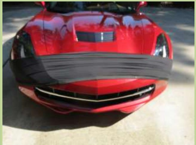
Step 7 may appear confusing until you read the text and then look at this picture. The outside bottom corners will not stay on the edge of the bumper. As noted in the instructions, this next step is optional but recommended. The instructions indicate the bolt that holds the outer edge of the air dam just be loosened to provide a gap for the Bra to fit into. I found it required several turns to provide the needed gap. I was concerned the screw could work loose, especially when not using the Bra..
