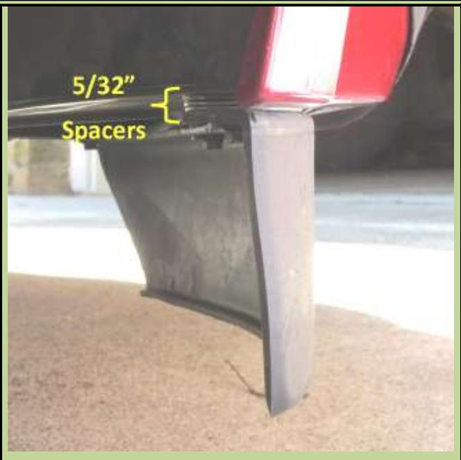
This is a picture with the Bra corner inserted into the gap between the bumper and the air dam. Looks like it will hold fine. Will must see how well it holds at high speed.
