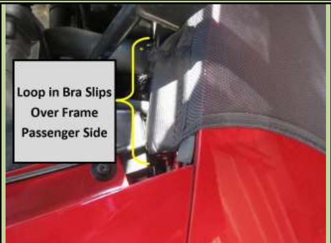
Although not mentioned in the Instructions, I was able to place the "Plastic Cover" back over the Bra loop. It does fit in with friction as noted in the instructions. Note on the passenger side there is a cable that fits over it and helps it stay in place. Since I will only be using the Bra for long trips I might leave them off until I remove the Bra
