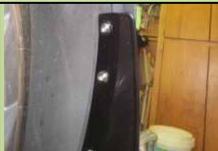
These are the three snaps used to hold the Stage 3 winglets. They are recessed but there is room for the male snap on the bra.
