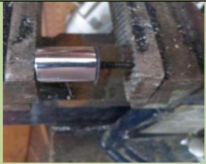
The washer will deform slightly but one blow from a hammer on the vise anvil quickly flattened it. It slipped over the supplied snap without having to ream out the hole.
