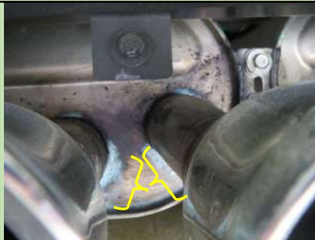
This picture was taken after a few brush strokes were made over the rusted area. Two areas are marked in yellow. The milk like, somewhat foamy reformer looks light blue in this picture as well as the one below. It is best to put on some light coats than come back and repeat in a few minutes.
