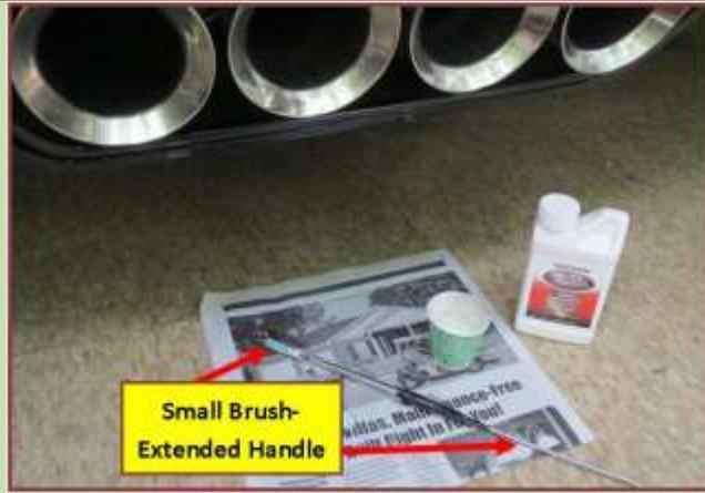
This is what was I used to gain brush access to the back muffler panels and welds. A small metal handle disposable brush was taped to a small rod so access to the rusted areas could be made mostly from the rear. No reason to jack up the car just lay on your side. A small amount of Rust Reformer was placed in a paper cup. You don't need much. It is indicated the product has a shelf live and it should be not used after about a year.
