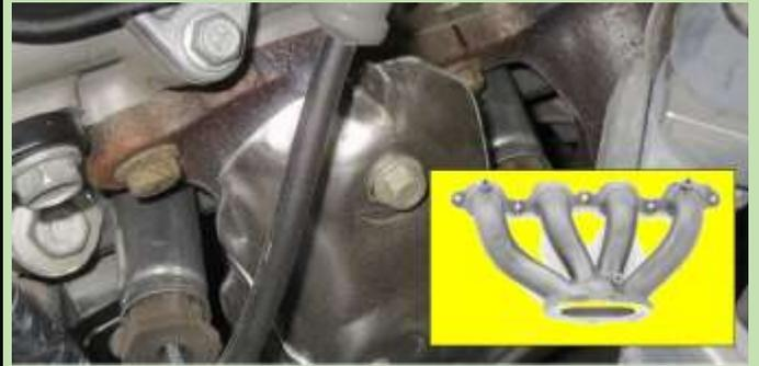
Rust Reformer as applied. As with the muffler it goes on very easy and you don't worry about brush strokes or getting some on non-rusted parts once dry. It does not show on non-rusted areas. Made the long-handled brush as before to gain access to all on the visible exhaust manifold areas on the driver's side.
