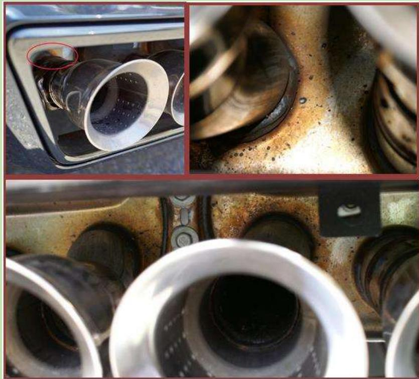
large pipe welds and weld spatter that no doubt melted the thin aluminized surface exposing uncoated places of 409 stainless that quickly starts to rust.
