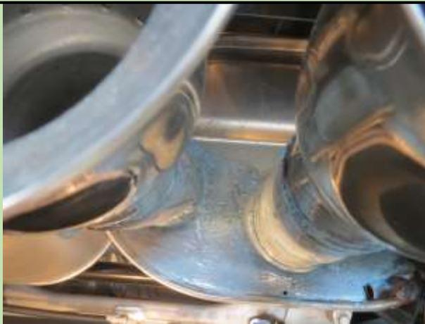
Rust reformer applied with a brush taped to a dowel. Mostly all from the rear. It took less than 10 minutes.
