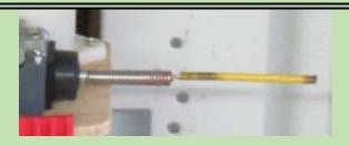
To assure the metal probe does not scratch the mirror, if it ever hits, it was first dipped in liquid plastic. Then a piece of yellow vinyl shrink tubing was placed over the coated wire, extending 1/8 inch past the end. A heat gun secured it to the coated probe.
