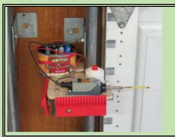
This is the finished assembly with the battery pack in the "vegetable can" holder screwed to the platform! Not quite an Andy Warhol picture but it works. The battery pack can be removed when needed, which hopefully will be seldom.
