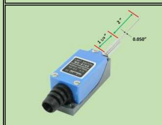
The limit switch selected is a model TZ-8169, a SPDT switch that has a thin, 0.050-inch diameter, 2-inch-long probe wound into a spring that is 1 ¼ inches long before entering the switch. It has both normally closed and normally open terminals. The device only uses the normally open contacts which close if the probe is touched by a mirror.
