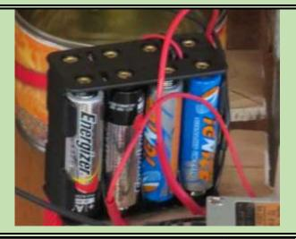
To supply the 12 volts needed for the alarm buzzer, a holder for 8 AA batteries is used. It was less than \$4 on eBay.
