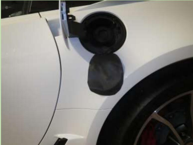
The gas bib for the C7 Corvette attaches to the bottom screw of the ring cover in the fuel door recess. I also placed a washer between the bib and the screw head.
