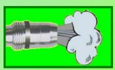
Depending on the number of weld starts, tack welds and how often the MIG wire is just inched to cut of the end or position it in the joint, the gas surge at the weld start can waste over half the shielding gas used!
