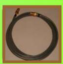
delivery hose from gas supply flow control, to welder. It uses a small inside diameter hose that holds only about 20% of the stored shielding gas, therefore saves 80% of the gas waste at each weld start. It includes a special flow control orifice in the brass fitting at the welder end to limit the peak surge flow to a rate that does not cause excess turbulence. Enough extra gas is available to quickly purge
