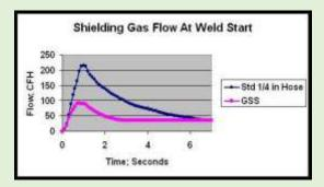
With a standard gas delivery system the surge flow rate is turbulent and mixes air into the shielding gas stream causing excess spatter and porosity. For this pressure piping application all welds must be UT inspected. The *GSS* restriction orifice eliminated problems caused by air in the gas stream and significantly reduced internal weld porosity at the start.
