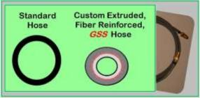
A simple way to significantly reduce shielding gas waste is to employ a shielding gas hose with a smaller ID.
