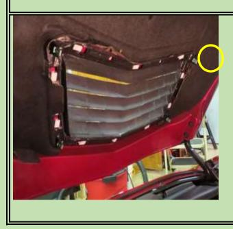
With the 10 clips in place, it's time to press them into the CF vent into the holes in the hood. I used a small screw driver to lift the insulation above the CF hood vent edge. This raised insulation edge will be hidden by the inner plastic cover. I used the side of my closed hand to tap loose clips into the hood.
