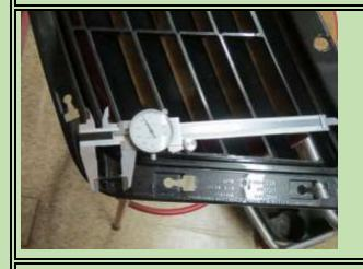
Before placing the CF Hood Vent on the car, check the size of the CF tabs that will hold the clips and inner trim cover. I found the OEM plastic vent had 0.9 inch wide plastic stands to which the metal clips were attached. The CF stands were wider. In fact some were wider than the slots in the plastic inner cover. Two were 1.125 inches wide and did not fit in the plastic cover slots.
