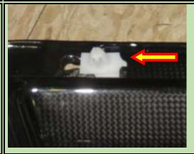
Note, there are thin rubber type washers that fit over the clips. They are probably used to stop rattles. They just slip over the clip tip.
