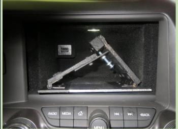
This is a picture of the assembly being placed into the cubby. The sides have not been raised to press on the roof.
