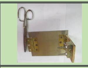
However, to maintain good access to the USB port, the left side was designed to wedge a piece of 1/8-inch aluminum upward into the roof. It was slotted so it could be made exactly the right height than secured with a bolt and nut.
