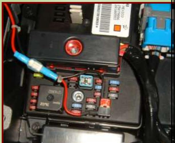
We accomplish that by using the “Add-A-Circuit.” Place the 10 amp fuse you just removed into the side of the “Add-A-Circuit” where the wire (red color for ours) exits the device. There is no fuse in the other side. One of the open female slots in the other side will be used to get power to our new switch.
