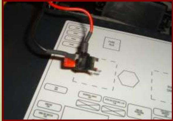
Now we must get the power back to the side of the fuse panel that powers the Dual Mode Control. It is one of the two fuse slots that are empty on the ‘Add-A-Circuit’. To get the power into that side; take the small male spade connector and using a pair of heavy wire cutters-(side cutters) shape the end to look similar to one side of the mini fuse. i.e. cut red area away as shown in photo.
