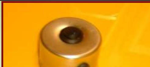
Now drill a hole into the side of the front cup holder! The hard part is psychological! Use an 1/8 inch drill bit at about 1:30 looking down from the top of the cup holder about 1 inch from the bottom. It will go through the rubber and plastic very quickly so don't go to fast. Once through, use a 5/16 inch drill to open the hole larger. That is large enough for the two # 16 wires that will be slipped through and some inevitable misalignment.
