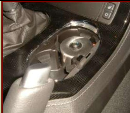
Now drill a hole in the side of the "Switch Holder" to line up approximately with the hole just drilled in the cup holder. Make it larger so there is room for a rubber grommet to protect the wires. The holes do not have to line up perfectly since there is a small gap between the "Switch Holder" and the side of the cup holder.
