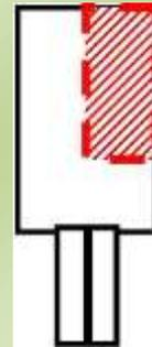
The cut spade connector will be connected to one of the two wires coming from the switch. It is inserted in the slot closest to the red wire which exits the “Add-A-Circuit.” Carefully look at the photo - it is the slot on the top. Don’t worry. If you pick the wrong slot you’re just putting 12V to the side that already has 12V and nothing will happen! It just won’t work!
