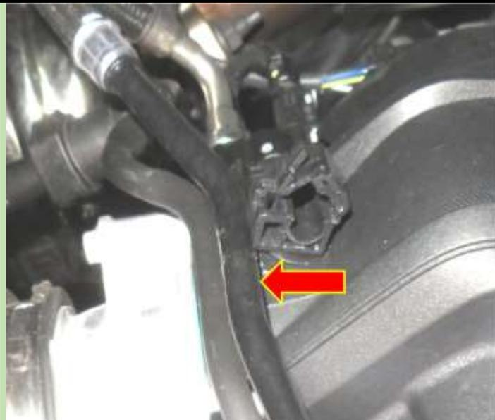
Place the hose in front of the engine cover out of the way. Best to keep the clip attached and remove it after. One of these "Professional Youtuber" videos showed removing it while the cover was attached. Bad idea! They took quite a while and needed several tools. In the end they hacked-up the plastic barbs that holds the clip in place and showed it was very loose when they reinstalled.
