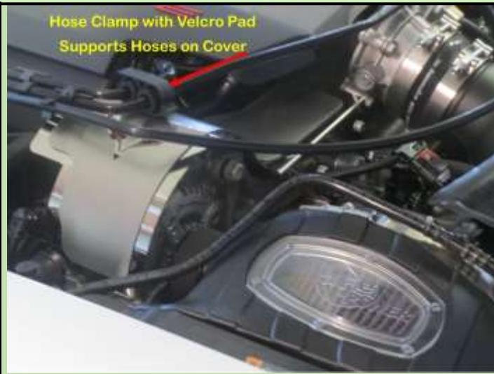
This is a finished pic of the cover installed. Looks great. The modified clap holding the two hard plastic hoses now has only Velcro in contact to the pad cover.
