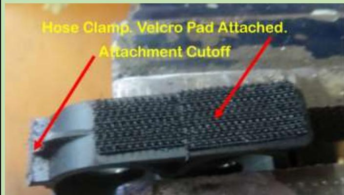
Decided rather than just discard the hose clamp, as recommended in the Instructions, I would use it to stop any rattling of the hoses on the alternator cover. This would only be an issue with a dry sump.
