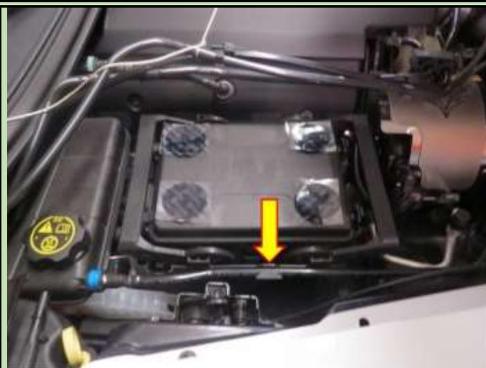
As suggested in the instructions placed the 4 pairs of Velcro as recommended in the corners. But was concerned as the top is NOT flat and would the Stainless Cover be able to press evenly on both sides?
