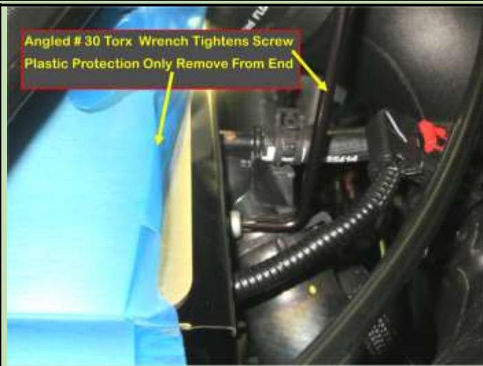
To remove the two OEM screws used the right angle Hex Tool # 30 Torx wrench. Did not need the extension I made, was able to get enough force by pulling on the end of the wrench while holding the bottom with my other hand.
