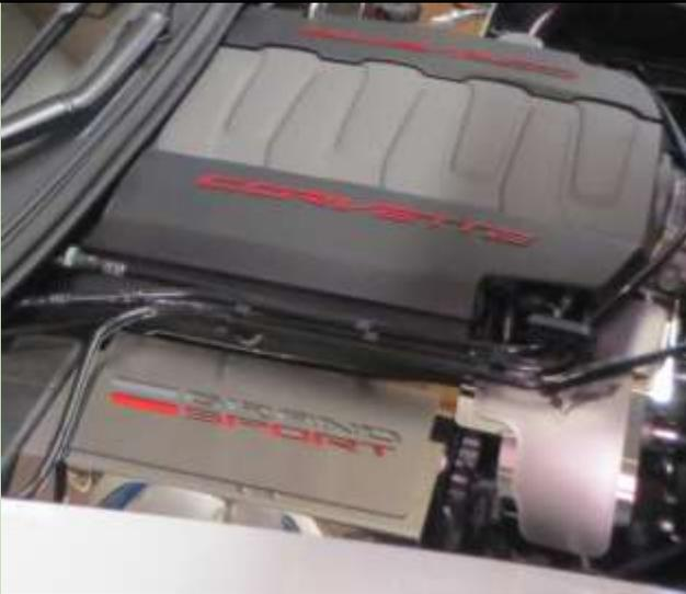
Pressed the cover down on the 4 Velcro pads. It held well. Would not try to remove the cover until the adhesive on the Velcro pads had a chance to fully harden.
