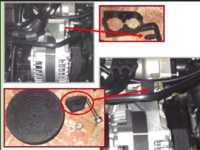
The hose clamp upper right in pic needs to be unclipped and removed. A large screwdriver can be used to leverage the plastic pin out of the hole in the raised boss.
