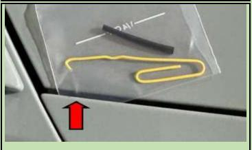
This is the "Hook" to grab the Stainless Steel Cable Loop in the open Hatch to Fender slot. Can grab either as the whole cable needs to come out.
