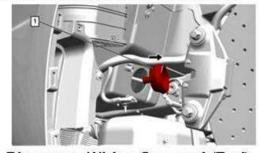
2. Disengage Wiring Grommet (Red)
