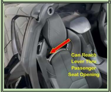
Ken thought thru every detail. Even mounted the cable activation switch upside-down so it can be operated from the open gap in the passenger seat!
