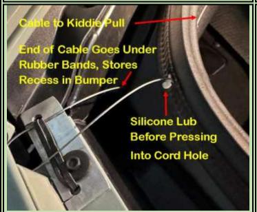
Had drilled a 5/32-inch diameter hole thru the Rubber Weatherstrip Molding angled down. Turned out it went thru two pieces of overlapping fiber like Trunk Liner that overlapped about  $\frac{1}{2}$  inch.
