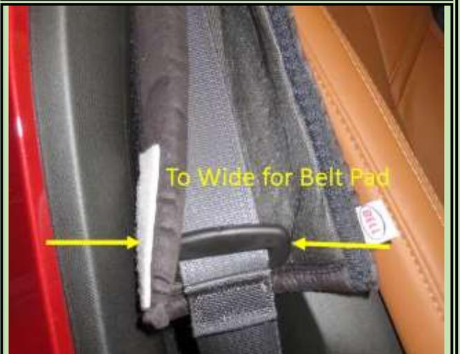
The solution was to add an inch wide piece of Velcro to the outside edge of the existing Velcro strip on the pad. A piece 3 inches long would provide the attachment interface needed. The added Velcro had a very strong adhesive tape on to the back side, designed to attach to material such as the foam from which the pad was made.
