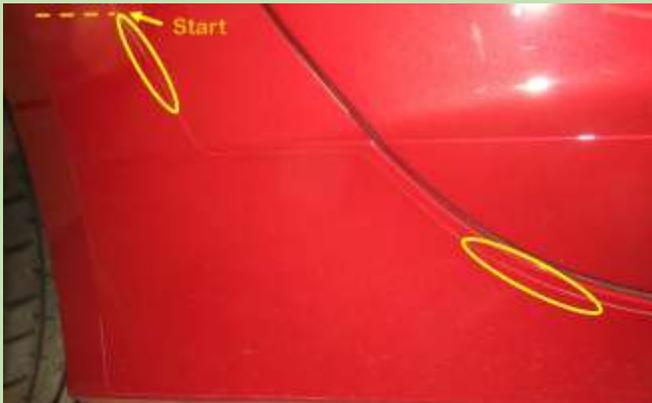
When I got my 2014 C7 Z51 saw GM understood the problem with the Coke Bottle shape and tires throwing rocks. They installed clear Protective Plastic Film (PPF) from the center of the door up to the front of the rear wheel wells. Pic Left. Highlighted with outline in Pic Bottom
