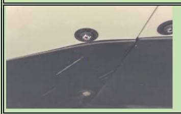
When I got home, looked. The mini splitter was fine no scrape. BUT the aero panel behind and two of the black screws holding it in place had a slight scrape! Also a scrape in the plastic seen as the white line. A none issue BUT
