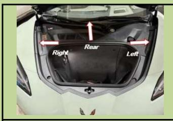
The Frunk has 3 Plastic Covers that must be removed to access the battery as well as the Lift Reservoir. The two side plastic covers must be removed 1<sup>st</sup>. Then the rear panel covering the battery, lift reservoir fill cap etc. can be removed.
