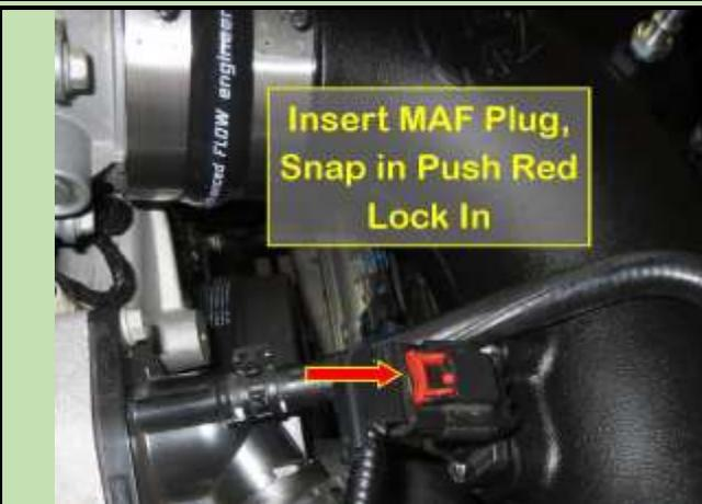
Next step is to install the MAF plug. Simple to do if you did not remove the red blocking clip, as I did! Just push the plug into the MAF socket you installed and then push-in the red blocking clip. The red clip just prevents access to the black tab below that secures the plug in the socket.
