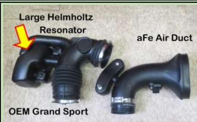
A Helmholtz Resonator in the intake tube forces air coming back out of the engine to slow down to fill the cavity, thus expending a great deal of its energy.. **Since these pressure waves are essentially sound, giving them a place to expend their energy before exiting the air filter box ends up dampening the intake noise and quieting the engine.**
