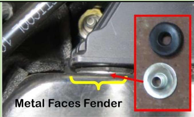
View of the OEM filter housing attachment. As with the C7 install this is one step that can be missed. Note the metal part of this fitting is facing the fender. When the *aFe* filter housing is installed, the metal part faces the engine and rubber touches the fender.
