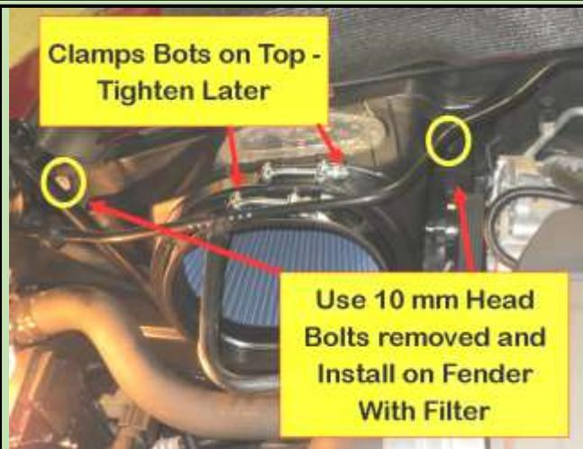
Note: pic is the new filter box after install. Now loosen all clamps on the OEM duct and remove it. Then (as shown here on the new filter housing) remove two 10 mm bolts that hold the air cleaner and its case to the passenger fender. To remove it, there is a plastic line for the radiator overflow going over it, which must be raised. I also removed that line from a clip on the left so it was easier to raise. You'll have to tilt the air cleaner assembly several ways to get it out.
