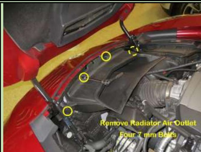
First thing to remove is the duct that takes air from 1/3 of the radiator and ducts it out the hood vent. This is straight forward, you'll need a 7 mm socket and a ratchet. You can use a long extension to remove the two center bolts and the one on the driver's side. But a short one or hand ratchet is needed for the passenger side. **There is a bolt in the center but it is not holding the air duct, so don't remove.**
