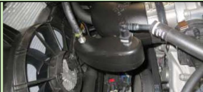
Next install the crankcase air intake hose on the hose barb (right hose in pic.) I have an Elite Clean Air Separator hose coming from the dry sump tank that just uses the open end of the hose slipped over the barb. So installed it with a constant tension hose clamp. Left in pic.
