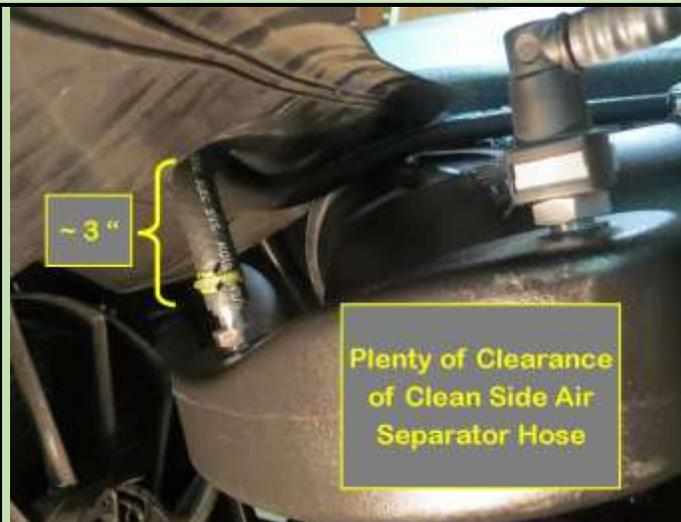
Was not sure how much clearance there was going to be between the *aFe* location for the clean air separator hose and the OEM air duct. Had thought if needed I could cut the original right angle hose end (like the one on crackcase the air inlet right) perhaps with a 6 inch long section of the plastic hose and silicone it into the ID of the hose and secure with a hose clamp.
