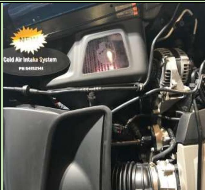
At the 2017 SEMA Show GM High Performance announced a low restriction air intake similar in appearance to the *aFe*. It's a similar appearing system to *aFe* with a plastic window to check for filter dirt.
