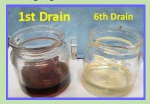
A forum Post reminded that the C7 is similar to the C6 and some prior Vettes. The clutch fluid gets dirty with use! The dirty fluid has been reported to cause the clutch pedal to be:
