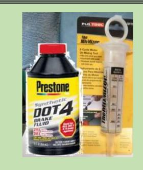
The small clutch fluid reservoir cap is labeled DOT 4, which is the fluid recommended. Be careful when you remove the cap, brake fluid will eat your paint! I put a towel around the reservoir and another from that towel draped over the fender so any drops would not touch the car!
