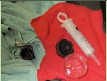
As a reminder, Brake fluid will remove paint! Note a towel was wrapped around the filler neck and another was placed on the fender.
