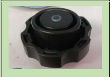
This is the cap with the extender pushed back the way it was found. The fluid level was filled to where it was found, ~ 1 inch from the rim.
