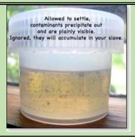
The general symptoms that can occur with "dirty clutch fluid" include a clutch pedal that becomes: Hard, • Soft, • Slow to return or lazy• Hung mid-way up or• Stuck to the floor
