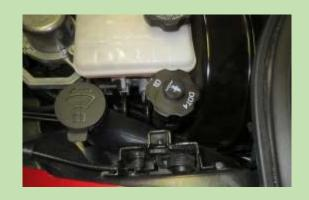
Procedure: 1) drained the reservoir with the syringe; 2) filled with new DOT 4; 3) depressed the clutch 30 times; 4) repeat as needed. That circulates the fluid so it mixes with the fluid in the line and slave cylinder. New clean fluid is mixed with old dirty fluid.
