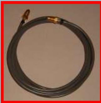
However to flow shielding gas though the welder and torch typically requires 3 to 5 psi depending on restrictions.
