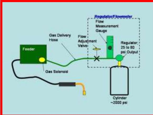
To keep flow at the preset level the gas pressure in the cylinder regulator will be between 25 and 80 psi. Flowgauge regulators (those with a flow calibrated pressure gauge) operate in this pressure range as well.)
