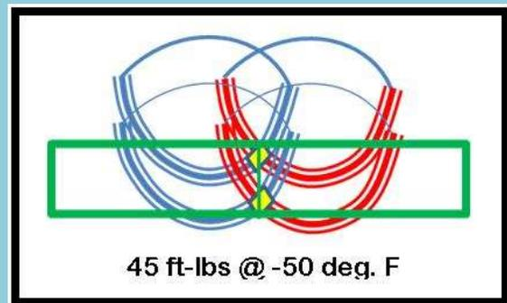
The above schematic shows the toughest Charpy in the series. It had double refined material (yellow area) at both outer edges of the specimen. It
