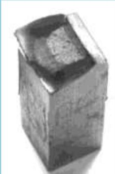
out, a Charpy specimen is subjected to triaxial stresses in the center while the outer edges have only one or two directional stress and strain. In ductile material these outer edges can experience significant deformation.
