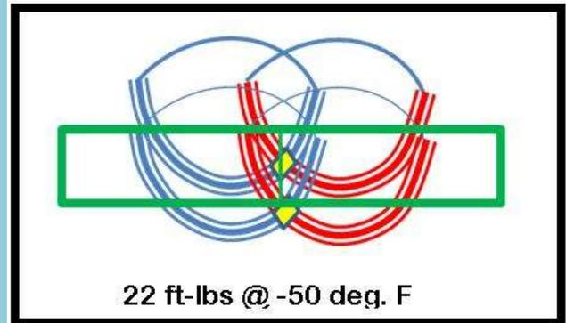
The toughness was somewhat higher at 22 ft-lbs. In general it does say that in this Mn Mo weld metal the doubly refined material is tougher than single refined material. It clearly shows that when the refined material is placed at the outer edges the toughness is significantly higher.
