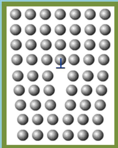
Dislocations are usually arranged in what are called edge and screw type and a combination of these structures. Sufficient to say for this discussion; as the material is
