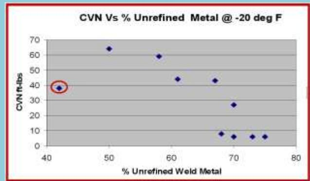
Again there is good correlation with the toughness and percent unrefined weld metal. Therefore the reheated area (HAZ) of the previous weld bead has a more refined metallurgical structure and higher toughness. There is one anomaly that as above will be explained in subsequent tests.
