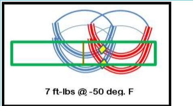
The above schematic shows the lowest toughness specimen produced. It had about 50% single refined material but that was placed in the center of the Charpy specimen or as Dr. Nelson would say most of the refinement was wasted! It matched the 8 ft-lbs in the prior process variations tests!
