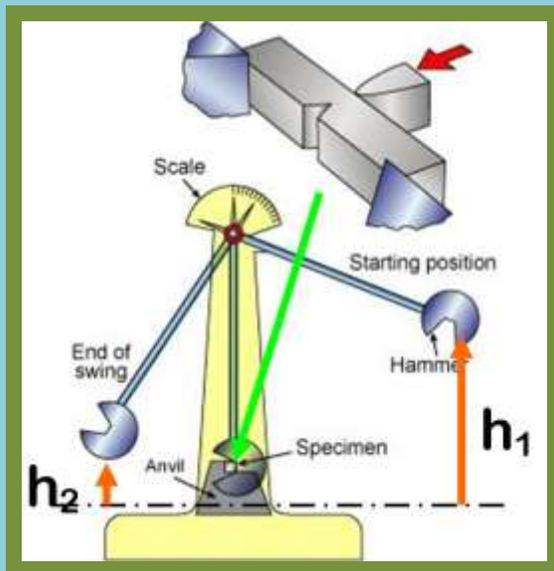
A precise “V” notch is placed in the bar. This can be ground or broached. The Charpy specimen is placed in a fixture such that the ends are held against a stop. A weight on a pendulum is raised. For example a 50 pound weight can be raised 3 feet (height  $h_1$  in sketch.) The weight is released and assuming very low friction bearings it will rise to
