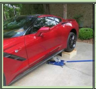
To have the C7 level, assuring all old oil is drained, wood "stanchions" were fabricated.
