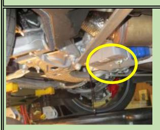
For my 2014 the oil cooler allowed room to use a 6 point 15mm socket on the drain plug and extension that fit under the oil cooler.
