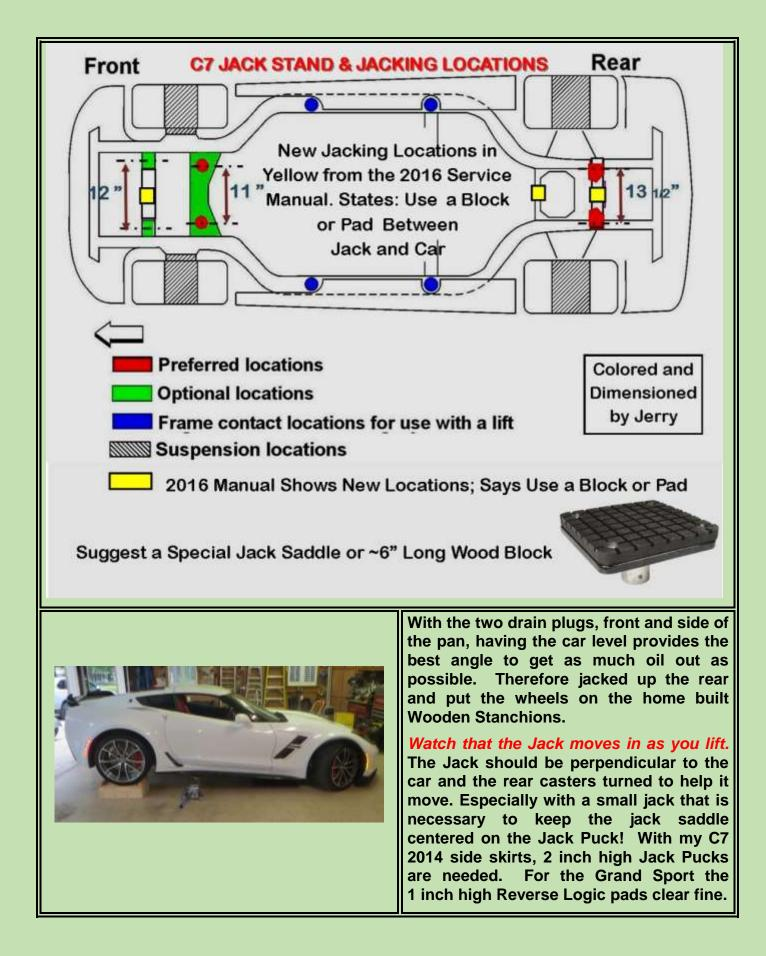
This is a view of the two jacks lifting the front on the 2 inch high Jack Pucks (red.) The Jack Stands were placed on the "Optional Locations" as noted on the GM chart. That left room for the drain pan and access to the front drain plug. The Jacks were left in place with no tension and plenty of room to access the side drain plug and oil filter. The stanchions can be seen below the rear tires.
