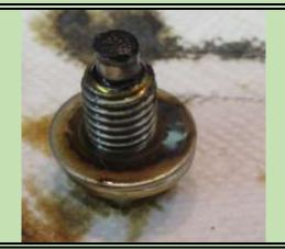
This is a pic of the drain plug removed from the front of the pan, on my  $2^{nd}$  oil change in the 2014 z51. That is the Drain Plug the one that drains the dry sump. Very few and very fine particles, cleaned with a paper towel. The longer magnet side plug was the same.
