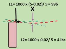
Considering only the top screw of the four used and since there is one on each end the 790 ponds max pull force X 2 = ~1500 lbs holding force so 1500/4 is a SF = 375
