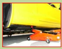
Photo left shows jack lifting left side of car.
