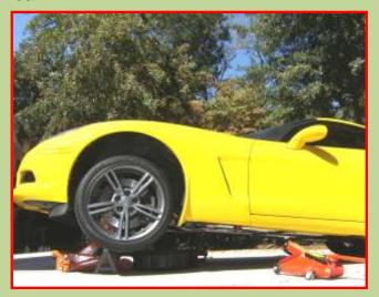
You can now remove the jack stands and lower the jack/cross brace several inches. Carefully crack the hydraulic opening valve. You can now raise the side jacks to reach the lifting pucks. Now remove the jack/cross brace from under the car.
