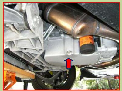
Now with plenty of room get a 14mm socket, and an oil drain pan and remove the drain plug. Red arrow shows the plug which is easy to access.
