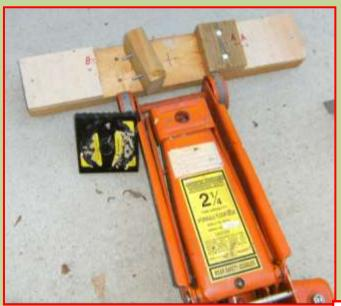
appropriate Jack Stands. Read all instructions that come with Jack Stands. When jacking the car put wheel chocks in back and in front of the wheels left on the ground.
