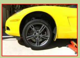
spoiler. Photo right shows about a 2 inch tire clearance that was all that was necessary to have the jack/cross brace clear the front spoiler.
