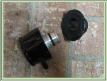
The "Clean Oil Separator is made in several parts but comes assembled. The plastic base screws in the same as the original oil cap. Then there is an "O" ring sealing the aluminum insert to the plastic base. These were difficult to separate in my case. In fact, a Forum comment got me to try.
