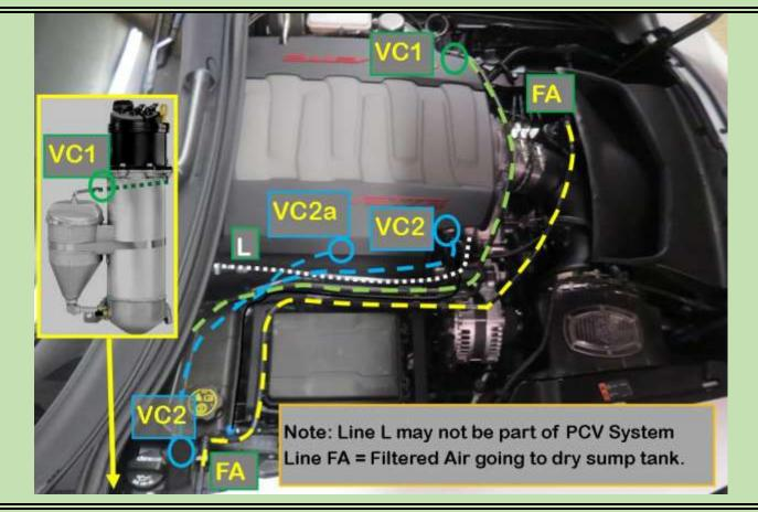
The Grand Sport has essentially the same PCV valve/hose arrangement as my 2014 Z51 (pic right.) It has a short PCV hose that goes to a passage to the intake manifold in a similar place as the 2014 C7 Z51.
