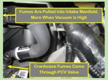
Tadge's comments about the dry sump reflect the different hose arrangement in my Grand Sport. In fact, it does have some ability to return some oil residue back into the oil reservoir. However the Grand Sport, although having additional lines and using hoses from the valve . ers to the dry sump tank <u>still has a PCV hose coming</u> from the crankcase and going to the intake manifold!
