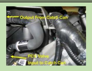
The 2014 Z51 had two hoses going to the air inlet tube, one to take fresh air into the crankcase, the other for burped air from the dry sump tank. The Grand Sport only has one. What does it do?
