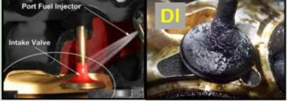
The Stingray LT1 engine has great performance. One reason is the higher tolerated compression because of more the efficient Direct Injection (DI.) Similar to a diesel engine; fuel is injected directly in the combustion chamber. However. this advance has a downside, there is nothing to help clean the oil residuals coming from the positive crankcase ventilation
