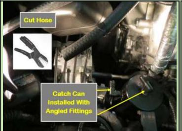
The "can" fittings were installed and aligned so the hose had a minimum bend. I used thread sealer. The hoses were cut to the length needed with an anvil cutter (a single blade razor could be used.) If you make them too long they could rub on parts as the engine moves when running. Measure twice and cut once, if too short, you're out of luck!
