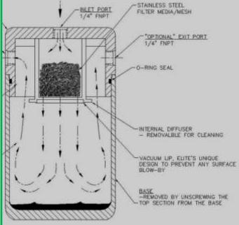
to condense before being sent on to the intake. For cars used as daily drivers the newer designs include a number of improved features. The picture upper right is the E2 model I purchased from Elite Engineering.
