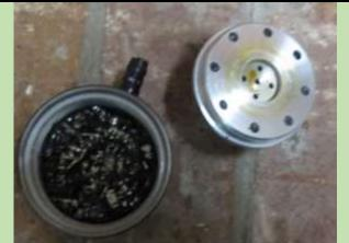
Cleaning the "Clean Oil Separator" This process is straight forward. The bottom machined aluminum baffle unscrews from the one-piece black top, as shown left. Pour some mineral spirits in the top over the stainless ribbon and watch it pour from the outlet hose barb. It will run clean quickly. When it runs out clear it's clean.
