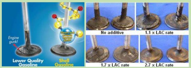
The picture left is from Shell and shows "coking" without their cleaning additive and a clean valve with it. The picture right shows "coking" without cleaning additives and with varying amounts added; 1.1, 1.7 and 2.7 units. As noted, it gets less with added amounts.
