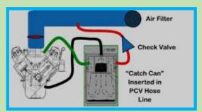
outlets, one outlet in the intake manifold (where the OEM PCV hose goes) and another added to a hole cut into the air intake tube. That requires a check valve OR air flow would occur from the line in the air intake tube though the "can" to the intake manifold and reduce any flow from the crackcase! *It was reported that they made an error on some shipments and the valve*
