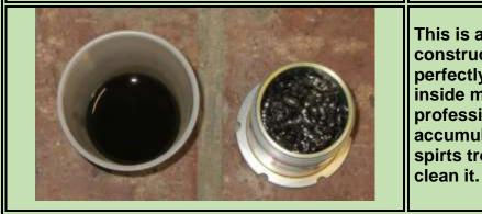
This is a top view. As with all the construction, the threads are cut perfectly and screw precisely into the inside machined top of the can. Very professional. Had there been more accumulation, would have run mineral spirts trough the stainless ribbon to clean it.
