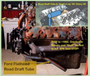
that "stuff" has to go somewhere, or it will build pressure in the crackcase. Prior to the 1960's it was common to use what was called a "road draft tube."
