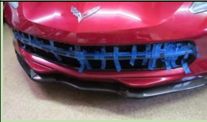
Did the same for the 2<sup>nd</sup> side with another batch of epoxy. The butted center fit perfectly. This time I put a somewhat larger amount on the wider part of the Overlay where it had felt slightly loose until I held it in place. As with the first side I put additional strips of tape along that whole section. It felt very secure, no need to hold it in place.
