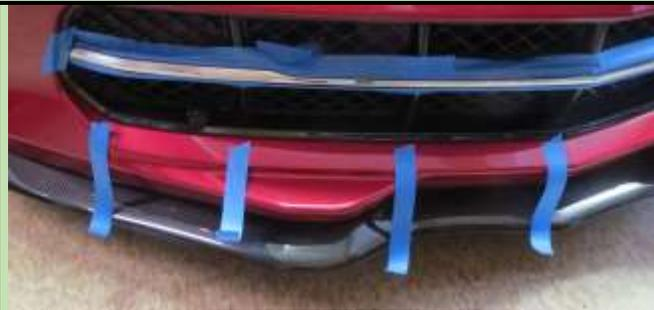
Prior to mixing the epoxy I placed strips of painter's tape where it would be needed to hold the Overlay in place.
