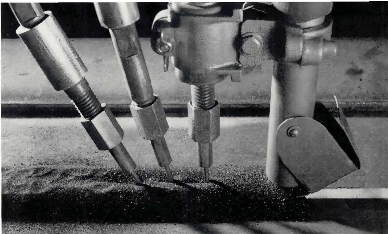
Three-wire submerged-arc welding under way, with motion from left to right
